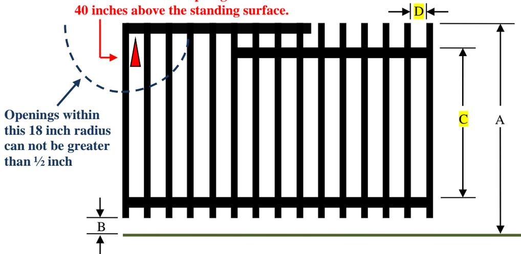
Dimension "A" must be 48 inches minimum from a standing surface to the top of the fence.
