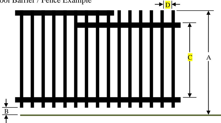
Dimension "A" must be 48 inches minimum from a standing surface to the top of the fence.
